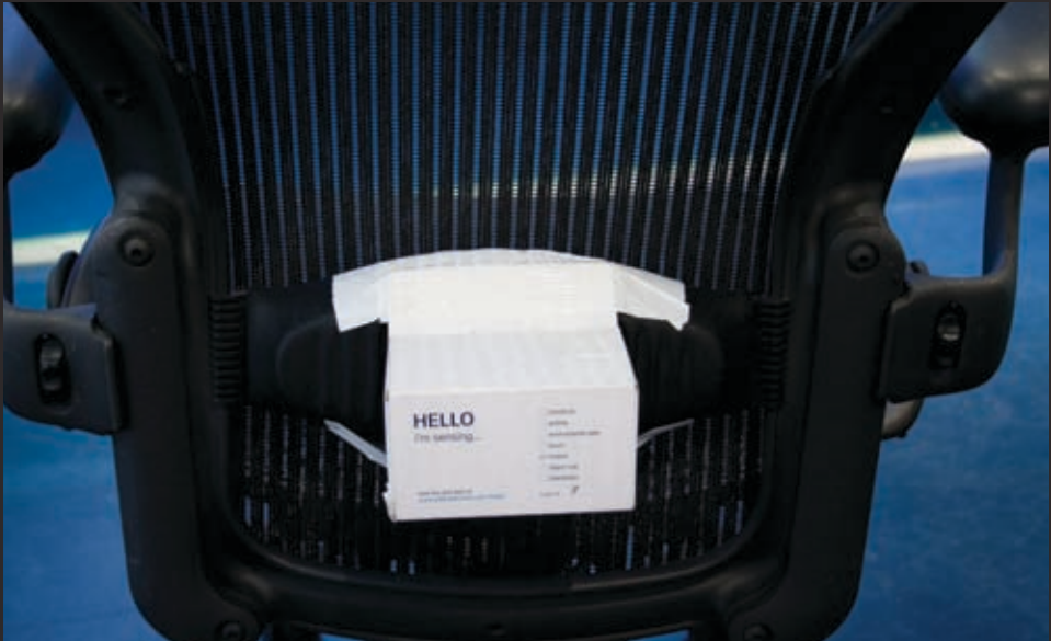
Accelerometers sensing fidgeting.
